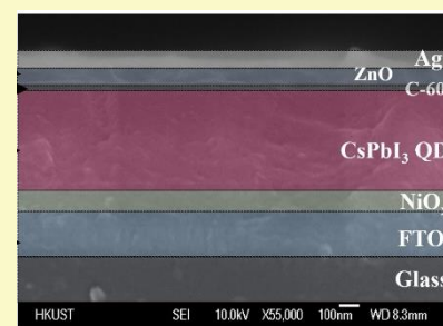
SEM cross-section of the device
